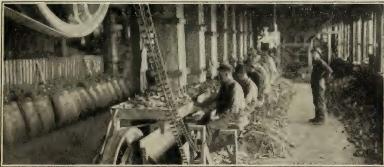
Carefully Butting and Tipping and Inspecting Each Ear Before Passing to the Sheller
